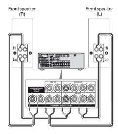
Connect the jacks on the Lo (or Hi) side of the front speakers to the SPEAKERS FRONT A terminals, and connect the jacks on the Hi (or Lo) side of the front speakers to the SPEAKERS SURROUND BACK/FRONT B/BI-AMP terminals.
